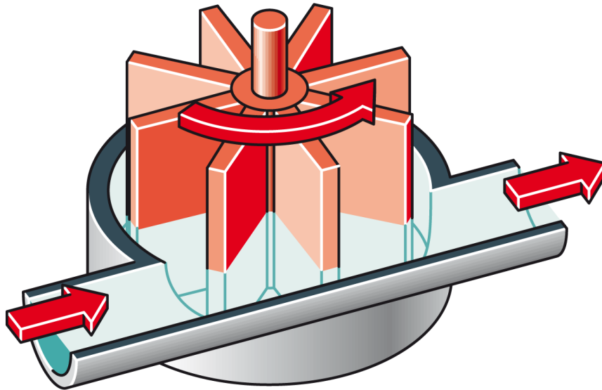
Figure 1: The internal structure inside a typical “velocity” water meter
